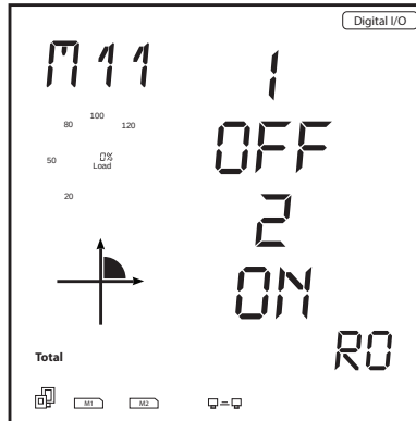
Figure 5-26 Relay Output Status Readings
