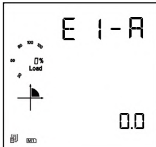
Figure 3-19 Energy 1 (To Generator) Display
